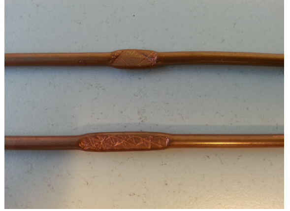
Fig. 7: The two faulty samples used for introducing soft faults in experiments.
