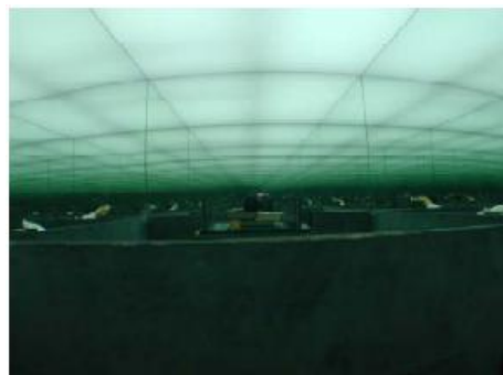
Figure 5. ‘Mirror box’ to simulate the artificial sky ( Maamari 2004)
