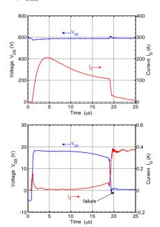
Fig. 5 Destructive test of C-MOSFET#1,  $R_G = 47 \Omega$ ,  $T_{CASE} = 25$ °C.
