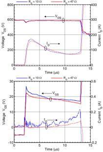
Fig. 7 Failure of B-MOSFET: drain and gate waveforms, at  $T_{CASE} = 150$  °C for  $R_G = 10$   $\Omega$  and 47  $\Omega$ .
