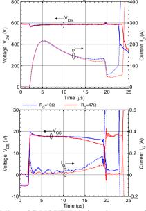
Fig. 8 Failure of C-MOSFET: drain and gate waveforms, at  $T_{CASE}$  = 25°C for  $R_G$  = 10  $\Omega$  and 47  $\Omega$ .
