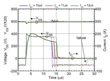
Fig. 9 Short circuit behavior of C-MOSFET for  $R_G$  = 10  $\Omega$  and  $T_{CASE}$  = 150°C.
