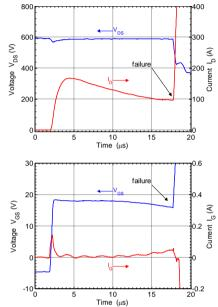
Fig. 4. Destructive test for A-MOSFET,  $R_G = 47 \Omega$ ,  $T_{CASE} = 25$ °C.
