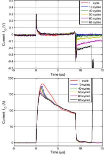
Fig. 11 Ageing of B-MOSFETs during repetitive SC,  $t_{SC} = 9\mu s$  repetition,  $R_G = 10 \Omega$ ,  $T_{CASE} = 25$ °C
