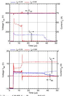
Fig. 3 Failure of BJT for  $T_{CASE} = 25$ °C.
