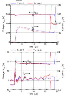
Fig. 6 Failure of A-MOSFET: drain and gate waveforms, for  $R_G = 10~\Omega$ ,  $T_{CASE} = 25^{\circ}\mathrm{C}$  and  $150^{\circ}\mathrm{C}$ .
