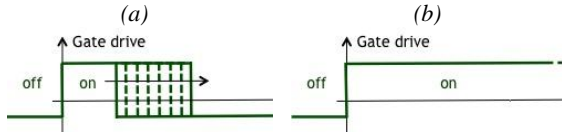
Fig. 2 Robustness tests under (a) short-circuit and (b) current limitation.
