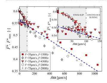
Figure 3. Maximum  $(F_{\text{max}}^*)$  and average  $(\overline{F}^*)$  dimensionless force as a function of the vibration velocity  $(A\omega)$  for different pulling velocity V and vibration frequency  $f[k=870\,\text{N m}^{-1}]$ . The red and blue lines correspond to quadratic and linear fit of the data, respectively (see text). *Inset*: zoom on the same data showing the transition between stick-slip (light gray zone) and continuous sliding (white zone).
