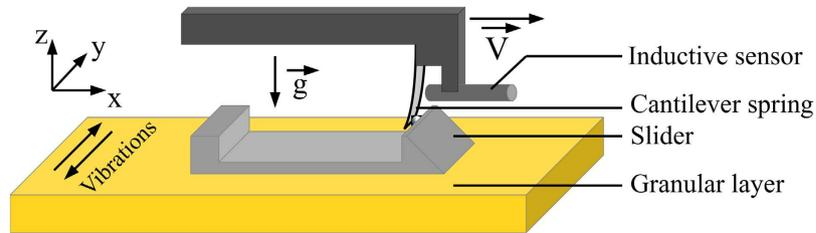
**Figure 1. Sketch of the experimental setup.** The slider is pulled at constant velocity, via a flexible blade, across the upper surface of a granular layer. A shaker (not represented here) imposes horizontal vibrations of the whole in the transverse direction (along the  $y$ -axis).
