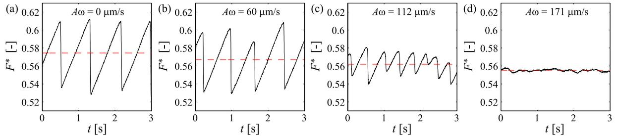
**Figure 2.** Dimensionless force  $F^*$  vs. time  $t$  for different amplitudes  $A$  of the imposed vibrations [ $k = 870 \text{ N/m}$ ,  $f = \omega/2\pi = 280 \text{ Hz}$ ,  $V = 35 \mu\text{m s}^{-1}$ ].
