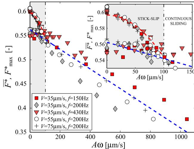
**Figure 3.** Maximum ( $F_{\max}^*$ ) and average ( $\bar{F}^*$ ) dimensionless force as a function of the vibration velocity ( $A\omega$ ) for different pulling velocity  $V$  and vibration frequency  $f$  [ $k = 870 \text{ N m}^{-1}$ ]. The red and blue lines correspond to quadratic and linear fit of the data, respectively (see text). *Inset:* zoom on the same data showing the transition between stick-slip (light gray zone) and continuous sliding (white zone).
