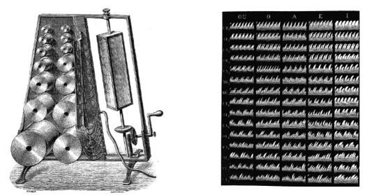
**Figure 4**. Kœnig's manometric flames analyser (left) and graphical inscription of the French vowels (/u/, /o/, /a/, /e/, /i/) "dancing flames" (right).
