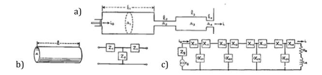
**Figure 6.** Dunn's theoretical model of vocal tract (from [27]). a) The 4 tubes approximation. b) The elementary cell corresponding to a cylinder of section A and length L. c) The complete model including the 4 elementary cells, an electrical analogue of the glottal source on the left and an electrical analogue of the acoustic radiation impedance on the right.
