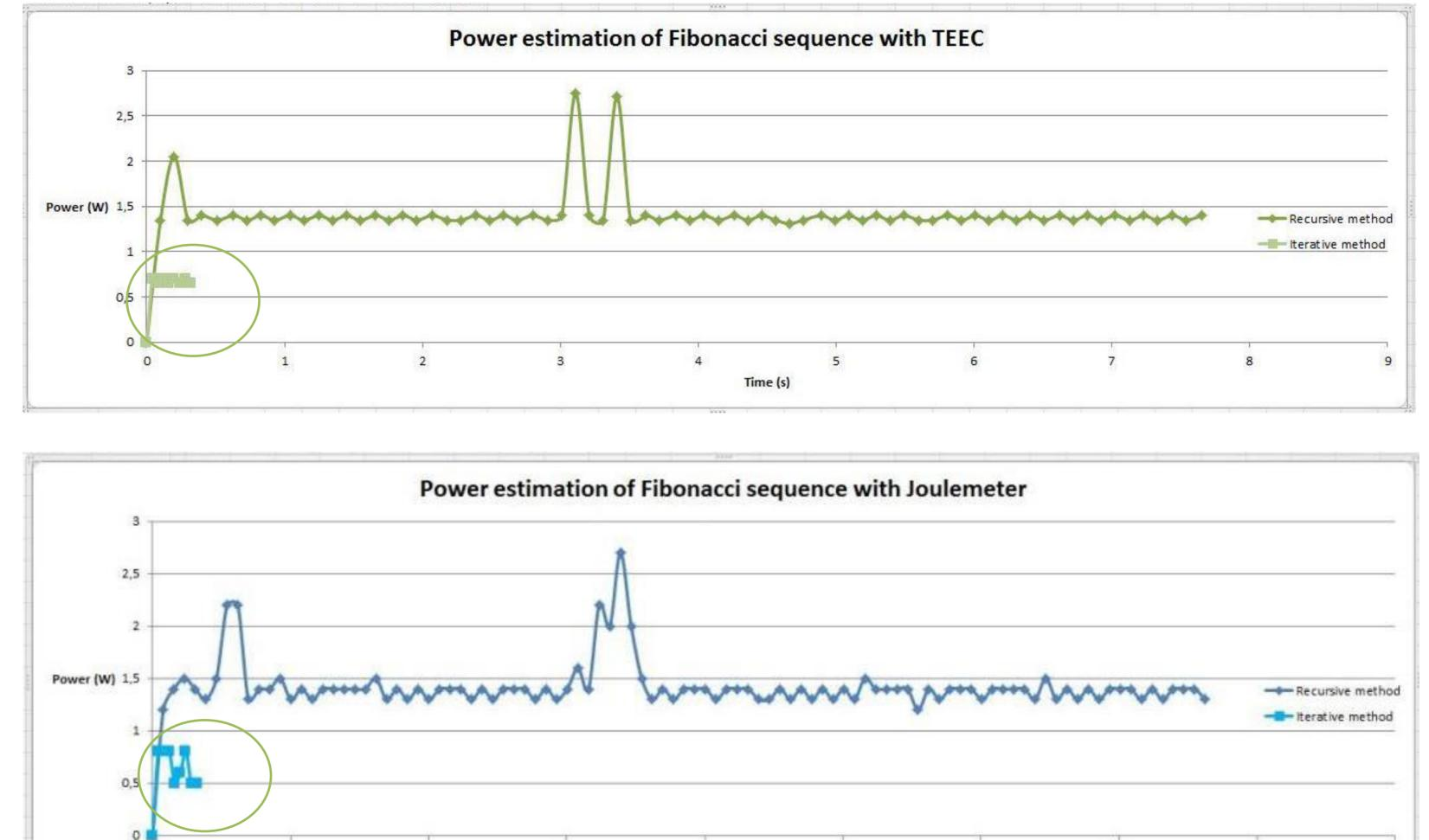
It is observable that quite similar results are obtained for the running application. It shows the effectiveness of the proposed tool and computational model, compared to Joulemeter.
