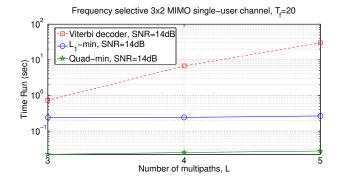
Fig. 6: Runtime evaluation of the proposed detector for SNR = 14dB, assuming BPSK modulation
