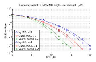
Fig. 3: BER performance comparison of the proposed detector versus the viterbi decoder and the [ $\ell_1$ -min] detector when L=4 and L=3.
