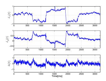
Fig. 5. Estimation of ocular artifacts and EEG using ICA with seven mixtures:  $e_x(t)$ ,  $e_y(t)$  and five EEG channels. The two figures on top show the ICs identified as "eye" components. The next figure is one of the ICs associated with the brain activity.
