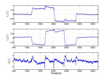
Fig. 4. Estimation of ocular artifacts and EEG using ICA with 3 mixtures:  $x(t), e_x(t), e_y(t)$ . The three estimated independent components are plotted: the two first one are related to the eye movements and the third one is the estimation of the brain activity.
