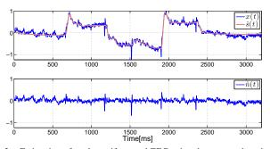
Fig. 2. Estimation of ocular artifacts and EEG using the proposed method. The figure on top shows the noisy EEG, x(t), and the estimation of ocular artifacts,  $\hat{s}(t)$ . The next figure shows the estimated remaining brain activity,  $\hat{n}(t) = x(t) - \hat{s}(t)$ .
