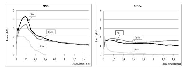
Fig. 4. Force-displacement curves for W/C = 0,65.
