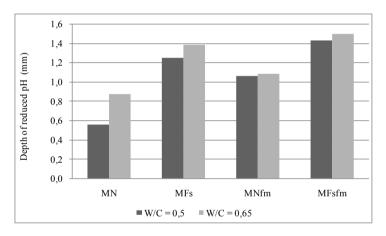
Fig. 5. Depth of pH change of the samples stored in sewers.
