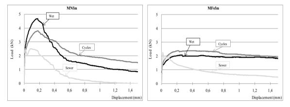
Fig. 3. Force-displacement curves for W/C = 0.5.
