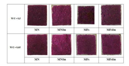
Fig. 6. pH modification detected by spraying with phenolphthalein.
