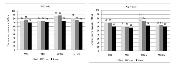
Fig. 2. Compressive strength of the mortars.
