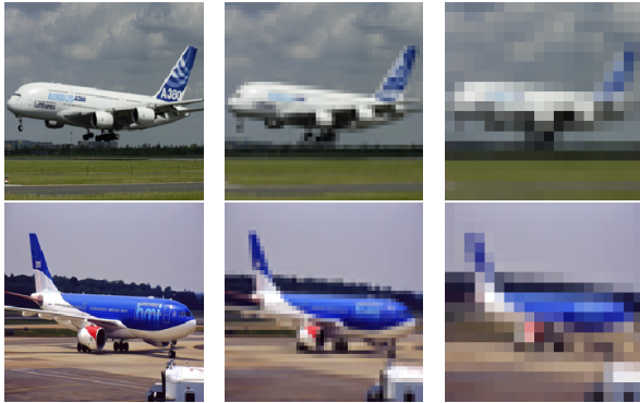
Fig. 4. Example of two Airbus airplane images (top A380, bottom A330-200) at resolutions 200 \times 200 (left), 50 \times 50 (middle) and 20 \times 20 (right). Resolution degradation occludes the discriminating details that enable distinguishing classes.
