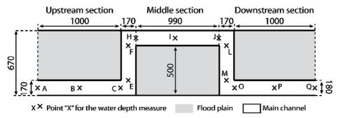
Figure 2: Plan view of the configuration used for the sinuous experiment. Dimensions in mm. The bottom elevation is nil in the main channel and equal to 0.1 m in the main channel.
