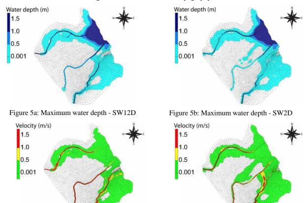
Figure 5c: Maximum velocity - SW12D
