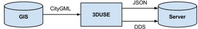
Figure 4: Pre-processing pipeline. CityGML files are prepared before being stored on the server.
