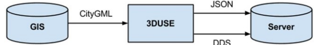
Figure 4: Pre-processing pipeline. CityGML files are prepared before being stored on the server.
