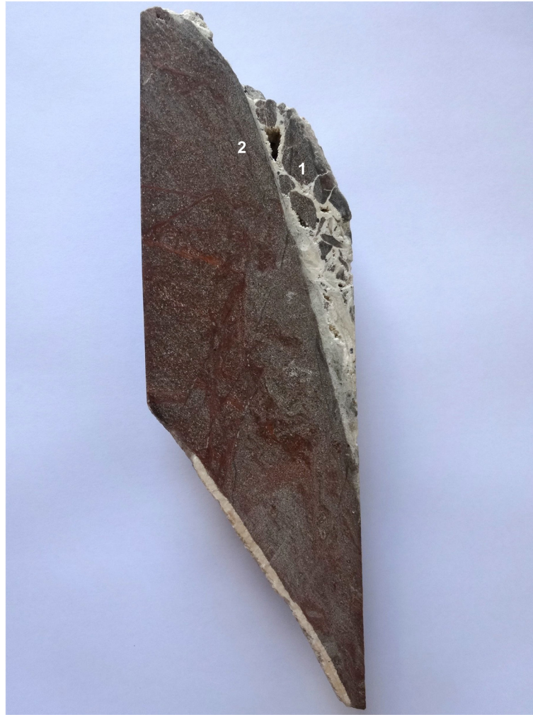
Figure 4 Core sample from a sandstone in the Buntsandstein at 1,204-m depth in the well EPS-1. The core sample exhibits a part of a fracture zone (1) and its damage zone (2). Barite and galena fill the hydraulic breccia. The diameter of the core sample is 8 cm.
