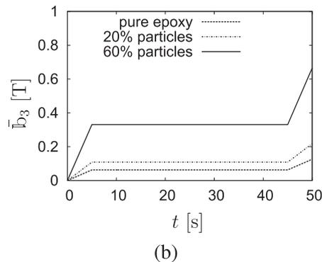
**Fig. 8.** Evolution with time of macroscopic magnetic induction in the 3 direction when a stepwise strain with time is considered and the evolution of the macroscopic field is (a) linear and (b) stepwise.
