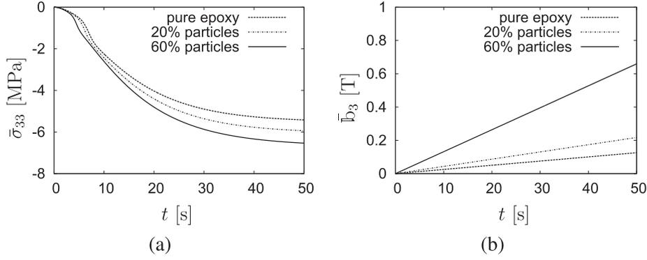
**Fig. 10.** Evolution with time of (a) macroscopic normal stress in the 3 direction and (b) macroscopic magnetic induction in the 3 direction, when the macroscopic magnetic field increases linearly and the macroscopic strain is zero. Shrinkage effects are taken into account.
