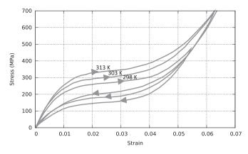
**Fig. 8.** Experimental isothermal uniaxial tensile tests at three temperatures: T = 313 K, T = 303 K and T = 298 K performed by Lagoudas et al. (2012).
