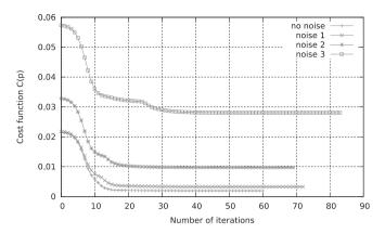
Fig. 7. Evolution of the cost function with the number of iterations for the four experimental data with various noise level.
