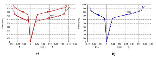
Fig. 6. Comparison between the simulated response and the experimental data a) for isothermal tests at the two temperatures utilized in the parameter identification procedure (323 K and 343 K). b) Experimental validation for an isothermal test at 333 K.
