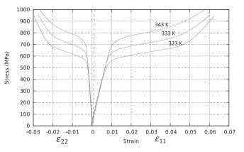
Fig. 3. Uniaxial stress-strain response of the NiTi superelastic alloy during three isothermal loadings.
