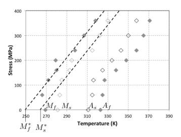
**Fig. 1.** Uniaxial stress-temperature diagram (from the isobaric experiments of Wu et al., 2003) that illustrates the difference of  $M_s$  and  $M_s^*$ .
