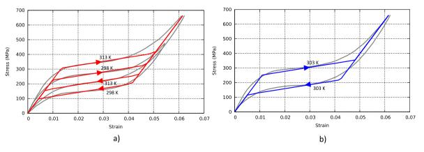
Fig. 9. Comparison between simulation using the identified model parameters and the experimental response in uniaxial tension a) For the two isothermal tests at the temperatures utilized for the identification (298 K, 313 K). b) at 303 K, temperature for the experimental validation.
