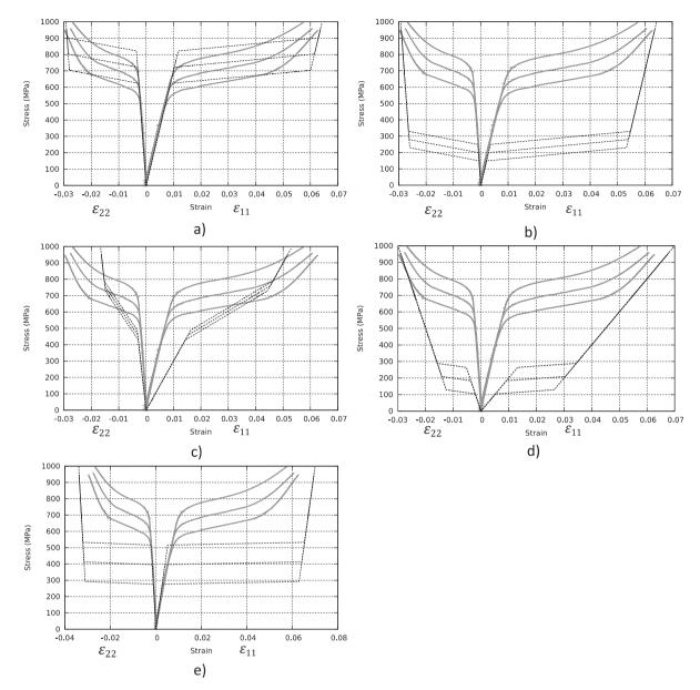
**Fig. 4.** Comparisons between the simulations (dashed black) of the uniaxial response using the initial set of parameters and the experimental response (plain gray) a) with the preliminary identification (Pl) b) with the parameters provided in Chemisky et al. (2011). c), d) and e) with arbitrary initial sets of parameters. All these initial parameters are summarized in Table 2.
