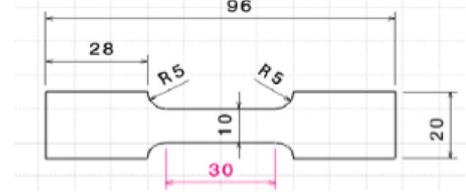
Fig. 2. Tensile specimen with 2.5 mm thickness.
