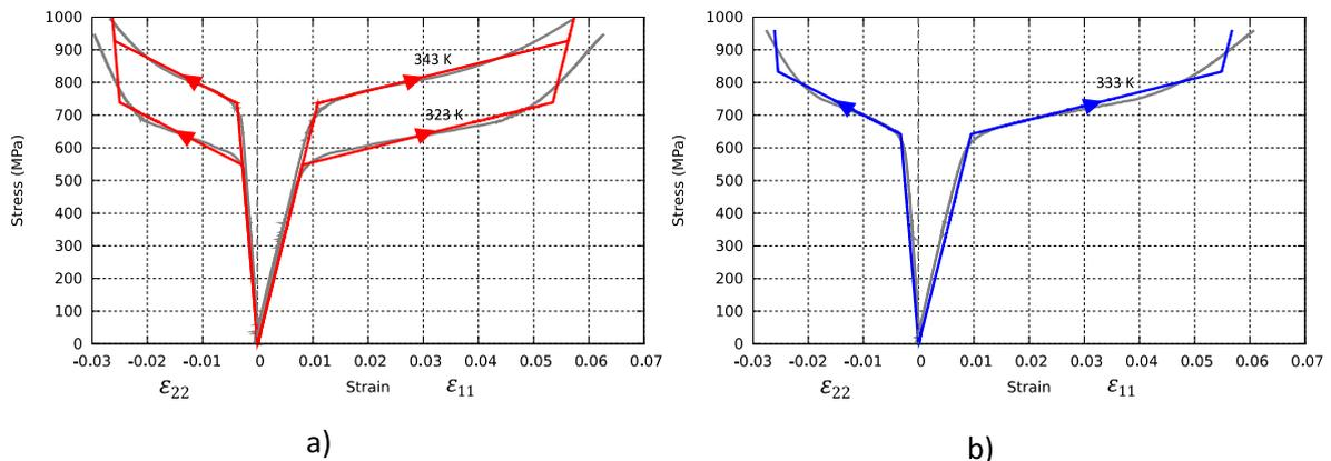
**Fig. 6.** Comparison between the simulated response and the experimental data a) for isothermal tests at the two temperatures utilized in the parameter identification procedure (323 K and 343 K). b) Experimental validation for an isothermal test at 333 K.
