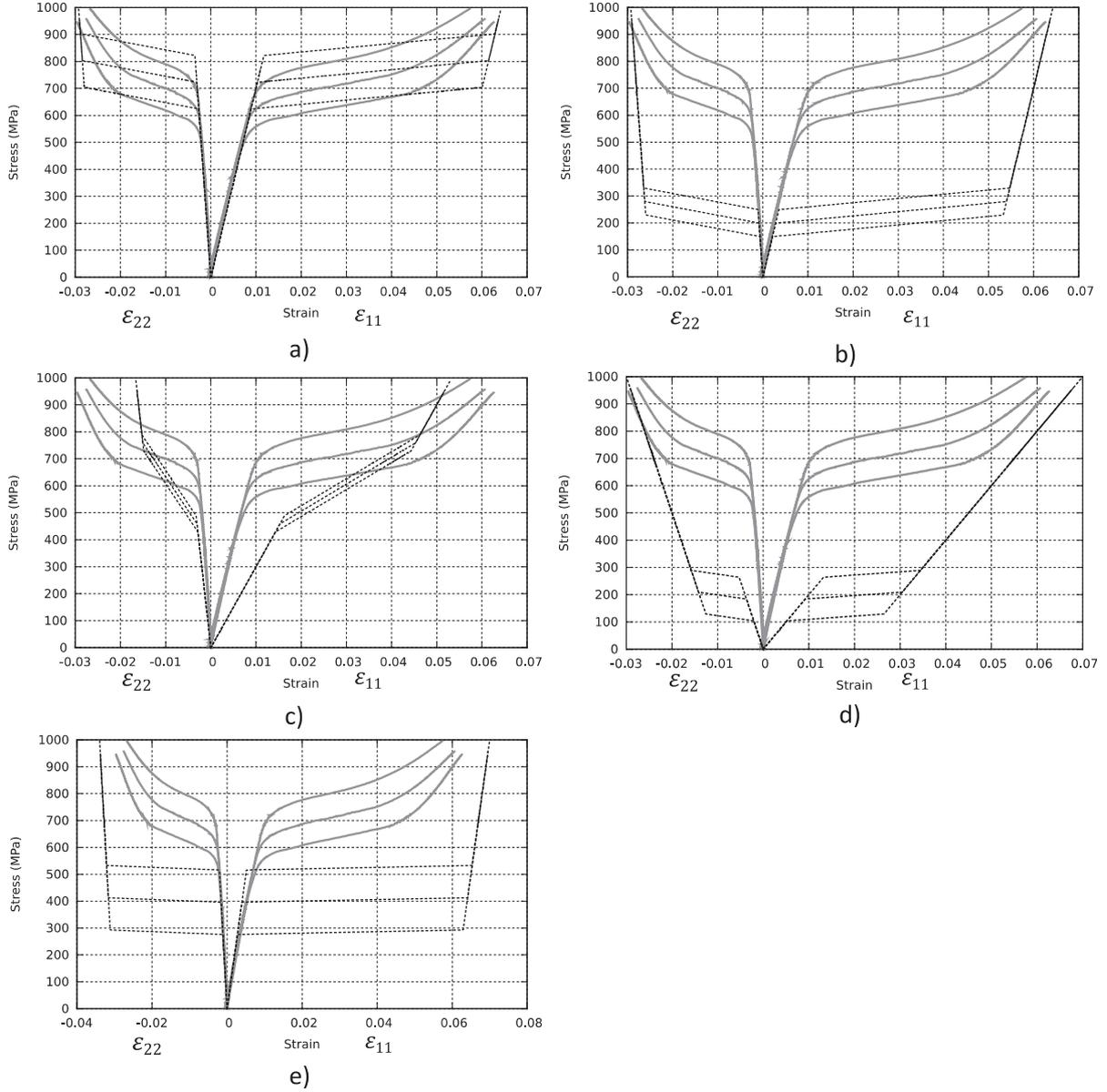
**Fig. 4.** Comparisons between the simulations (dashed black) of the uniaxial response using the initial set of parameters and the experimental response (plain gray) a) with the preliminary identification (PI) b) with the parameters provided in Chemisky et al. (2011). c), d) and e) with arbitrary initial sets of parameters. All these initial parameters are summarized in Table 2.
