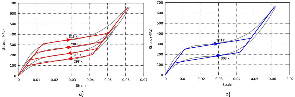
**Fig. 9.** Comparison between simulation using the identified model parameters and the experimental response in uniaxial tension a) For the two isothermal tests at the temperatures utilized for the identification (298 K, 313 K). b) at 303 K, temperature for the experimental validation.
