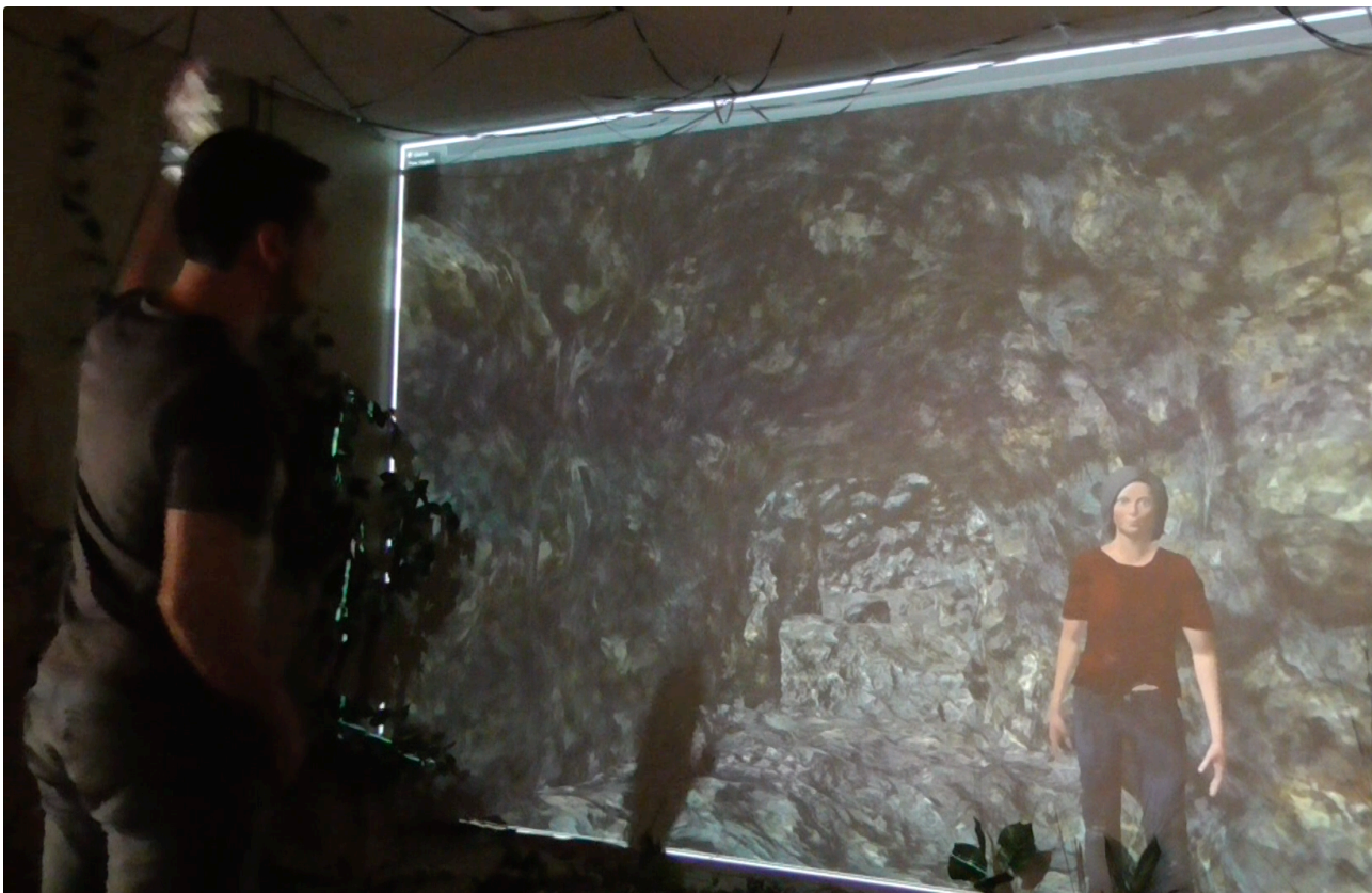
Figure 1. Human, interacting with ECA, performing a "hi-five" gesture. The human's gesture is sensed by a Kinect just in front of the projection wall and is interpreted via the gesture tool.
