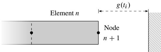
Figure 5. Rod approaching the rigid foundation at  $t_i$
