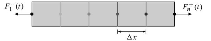
Figure 3. Boundary forces acting on the rod
