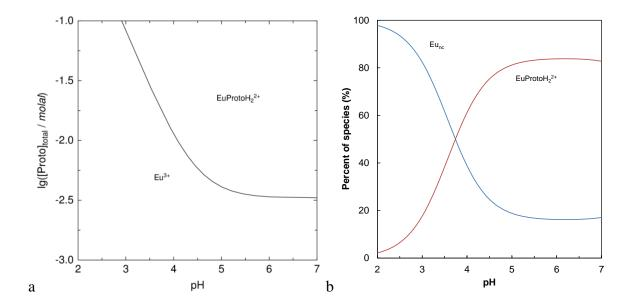
Figure 4. Predominance plot of the Eu(III)/Proto system at  $[Eu(III)] = 10^{-4} \text{ mol.L}^{-1}$  and  $I = 0.1 \text{ mol.L}^{-1}$  NaCl (a), and repartition plot of the Eu(III)/Proto system under EuProtoH<sub>2</sub><sup>2+</sup> hypothesis (b) – Eu(III)<sub>nc</sub> is defined in the text and SI.
