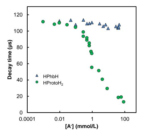
Figure 7. Decay time of Eu(III) at pH 5.5 as a function of ionized ligand concentrations (A stands for PhbH and ProtoH<sub>2</sub>,  $pK_a$  in Table 1): PhbH (triangles, [Eu(III)] =  $10^{-6}$  mol.L<sup>-1</sup>, I = 0.1 mol.L<sup>-1</sup> NaCl) and ProtoH<sub>2</sub> (circles, [Eu(III)] =  $10^{-5}$  mol.L<sup>-1</sup>, I = 0.01 mol.L<sup>-1</sup> NaCl).
