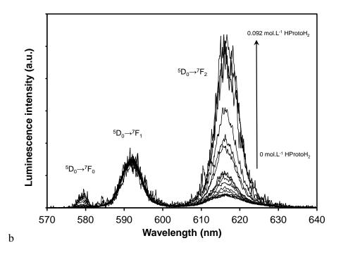
Figure 2. Normalized time-resolved luminescence spectra of Eu(III) complexed with HPhbH (a) and HProtoH<sub>2</sub> (b) the intensities were normalized to the area of the  ${}^5D_0 \rightarrow {}^7F_1$  transition for the sake of comparison;  $D = 10 \,\mu\text{s}$ ,  $W = 300 \,\mu\text{s}$ , [Eu(III)] =  $10^{-6} \,\text{mol.L}^{-1}$ ,  $I = 0.1 \,\text{mol.L}^{-1}$  NaCl, pH 5.5; The thick black lines represent uncomplexed Eu<sup>3+</sup>.
