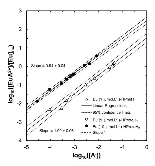
Figure 3. Determination of Eu(III) complex stoichiometries and formation constants from TRLS results using equation (2), at pH 5.5, [Eu(III)] =  $10^{-6}$  mol.L<sup>-1</sup> (empty symbols), and [Eu(III)] =  $10^{-5}$  mol.L<sup>-1</sup> (filled symbol), for EuPhbH<sup>2+</sup> (triangles, I = 0.1 mol.L<sup>-1</sup> NaCl), EuProtoH<sub>2</sub><sup>2+</sup> (circles, I = 0.01 mol.L<sup>-1</sup> NaCl).
