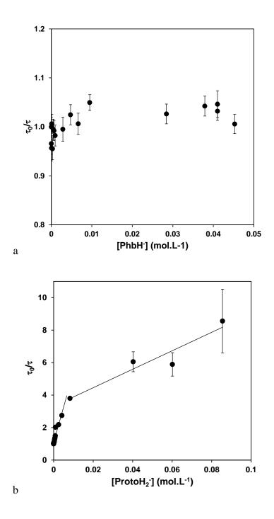
Figure 8. Stern-Volmer plot for  $[Eu(III)] = 10^{-5} \text{ mol.L}^{-1}$ , pH 5.5, for (a) HPhbH,  $I = 0.1 \text{ mol.L}^{-1}$  (NaCl), and (b)  $H_2\text{ProtoH}_2$   $I = 0.01 \text{ mol.L}^{-1}$  (NaCl). Error bars are  $2\sigma$  calculated from the propagation of error of the fitted  $\tau$  values
