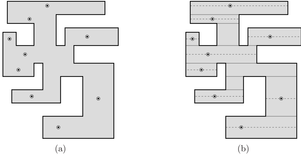
Figure 5: (a) A set T of terminals in a polygon P . (b) The decomposition \mathcal{D} of P into rectangles computed during step 1.
