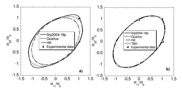
Figure 16. Predicted yield surfaces for AA6022 when the material parameters are identified, a) using the mechanical tests, and b) using the texture data and micromechanical simulations.
