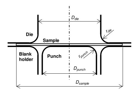
Figure 1. Cup drawing test geometry.
