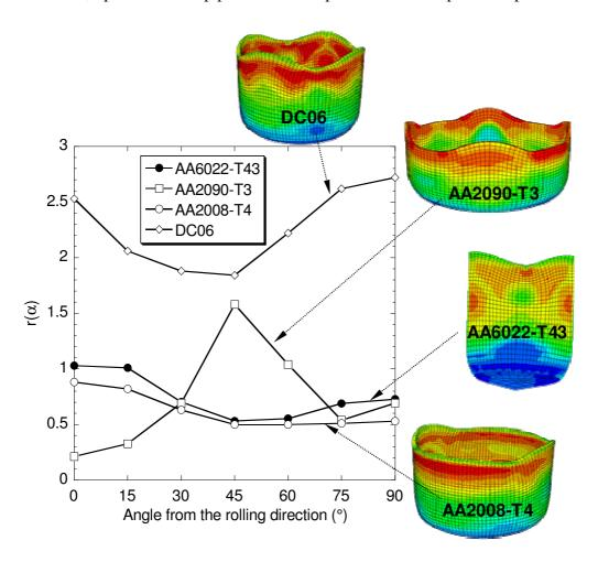
Figure 9. Experimental r-values and predicted cup heights for the different materials, using Srp2004-18p with material parameters identified by mechanical tests.
