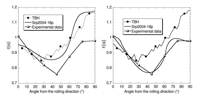
Figure 12. Impact of the identification technique on the predicted r-values for the Srp2004-18p potential and comparison to experimental and micromechanical results; a) identification using texture data, and b) identification using experimental data from mechanical tests.
