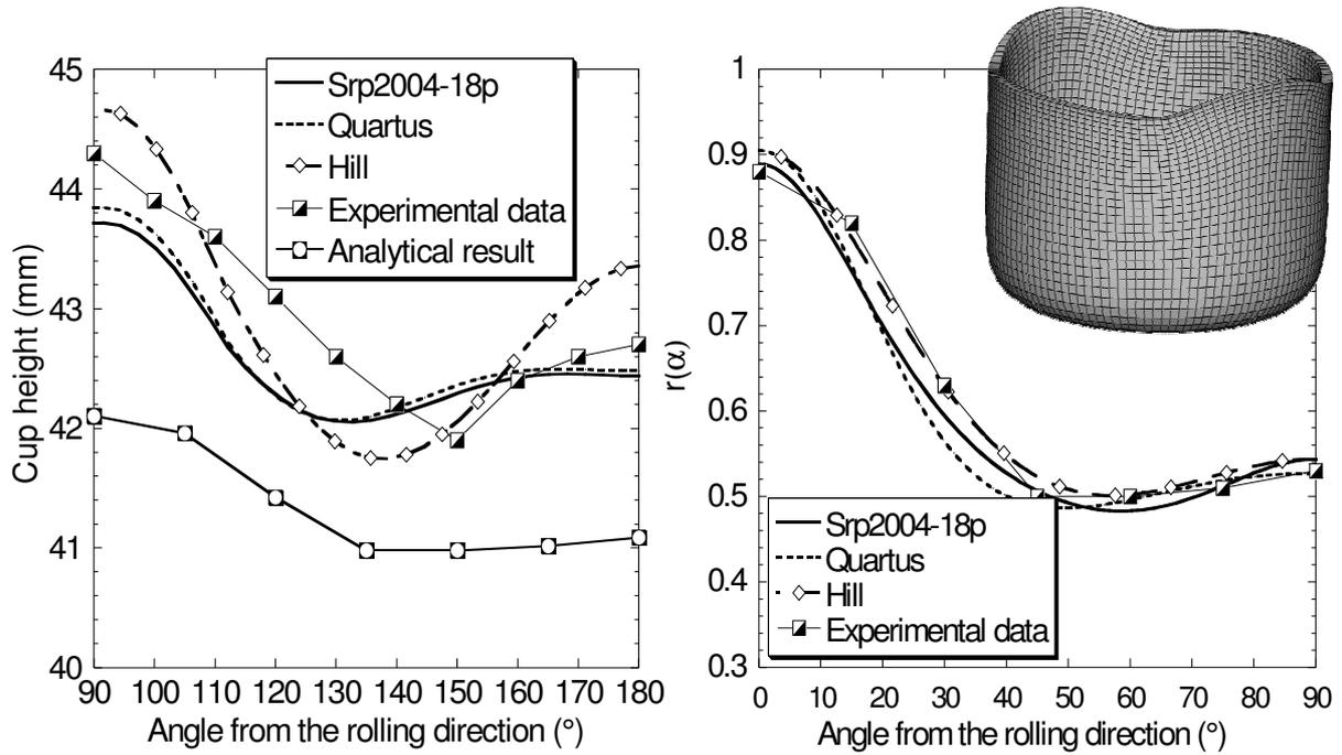
Figure 7. Cup height and r-value predictions for the AA2008 aluminum alloy.
