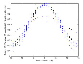
**Fig. 9.** Ratio of  $\partial F_X/\partial x$  evaluated with a 2-D model to that obtained with a 3-D model at 610 m downwind from the farm source (Site 1 in Fig. 1) as a function of wind direction. Each dot corresponds to a 30 min data point.
