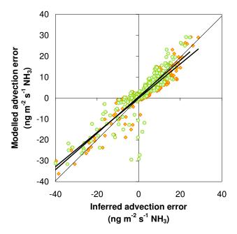
**Fig. 8.** Modelled versus inferred local advection error ( $\Delta F_{z,adv}$ ) at z=1 m and Site 1, estimated assuming a linear (orange diamonds) and a logarithmic (green circles) horizontal concentration profile. A linear regression between modelled and inferred local advection errors gives y=0.82 x-0.09 ( $R^2$ =0.88) and y=0.87 x +0.6 ( $R^2$ =0.76), for linear and logarithmic horizontal profiles assumptions, respectively.
