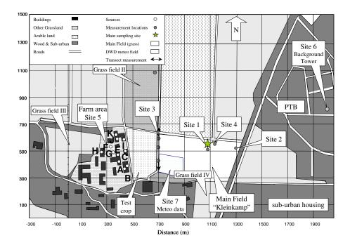
**Fig. 1.** Overview of the measurement site. The four concentration measurement locations used in this study are Site 1, Site 2, Site 3, as well as Site 6 where the background concentration was measured. The NH<sub>3</sub> source buildings are detailed in Sutton et al. (2009). Main Field is field I, and grass field II is the field where slurry was spread the 24 May 2000.
