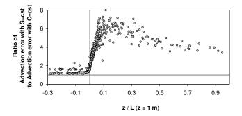
**Fig. 6.** Ratio of the modelled local advection error estimated with a constant surface source hypothesis (S=cst), and a constant surface concentration hypothesis (C=cst), as a function of the stability factor (z/L), where L is the Monin Obukhov length.
