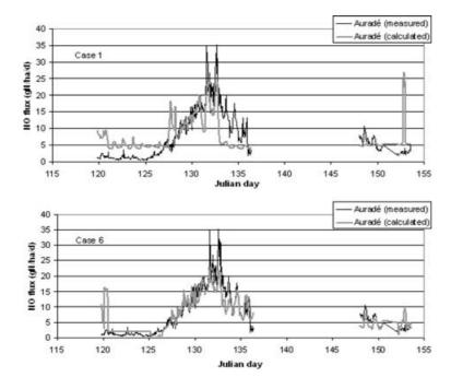
Fig. 3. Measured and calculated NO fluxes in case 1 (NO = f(surface temperature and WFPS)) and case 6 (NO = f(surface temperature and WFPS, deep soil temperature, fertilization rate, sand %, wind speed), function of Day of Year, for Auradé set only.
