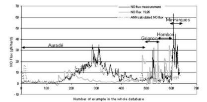
Fig. 4. Comparison between measured NO fluxes (black line), ANN calculated NO fluxes (dashed black line) and calculated NO fluxes with the YL95 algorithm (grey line), in gN. ha<sup>-1</sup>. d<sup>-1</sup>, function of the number of examples in the whole database. Each sub database is delimited by horizontal arrows
