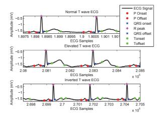
Fig. 4. ECGs after temporal features extraction
