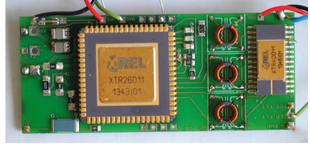
Figure 6: Picture of GaN driver board with 3 magnetic cores for signal insulation compatible with coreless transformers.
