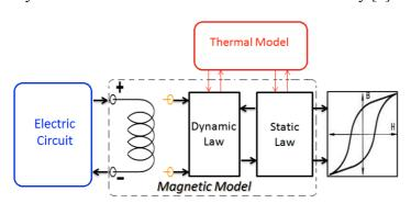
In the interest of precision and in order to be adaptable for different types of materials, magnetic magnetic the component model adopts structural modeling approach. As a consequence the model consists of 3 major blocks as shown adjacent figure: a responsible for coupling between electrical and magnetic domains using Ampere's and Faraday's laws, a static model to describe
