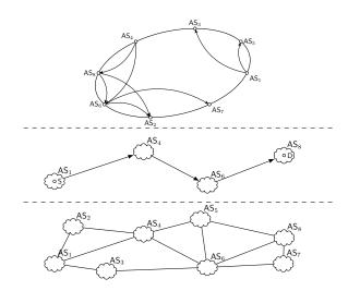
Figure 1. Network layers of our proposal. The first layer corresponds to the existing links between the ASes, the second one to the chosen path  $\prec S$ , D  $\succ$ . The final layer corresponds to the DHT organizing the score managers of ASes; AS<sub>8</sub> and AS<sub>6</sub> are the score managers of AS<sub>4</sub>, *etc*.
