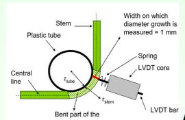
Experimental bending device which allowed to quantify the level of longitudinal strains during the stem bending.
