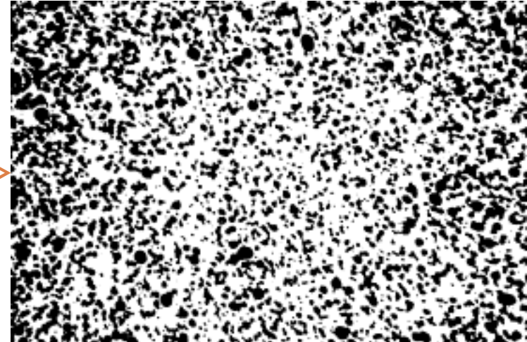
Segmented (binary) image of the UF-model cheese
