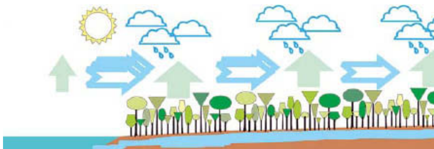
Figure 14. Biotic pump of atmospheric moisture: transpiration fluxes regulated by natural forests exceed oceanic evaporation fluxes to the degree when the arising ocean-to-land fluxes of moist air become large enough to compensate losses of water to runoff in the entire river basin. Source: Sheil and Murdiyarso 2009.
