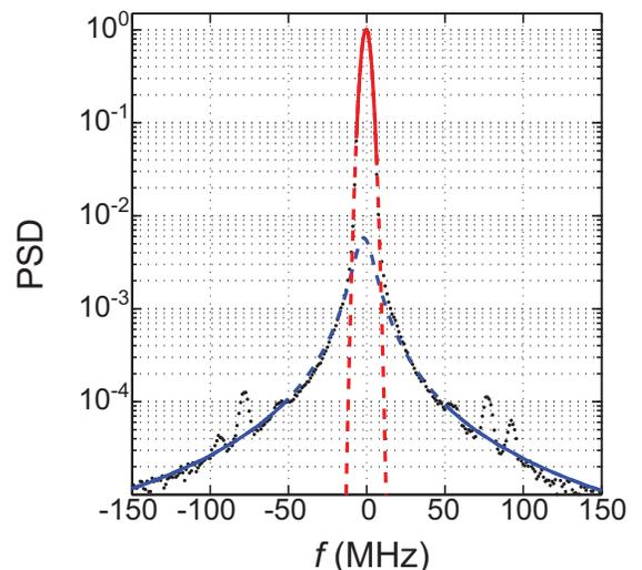
Fig. 7. Spectrum of the probe laser. The power spectrum density (PSD) of a beat-note signal with a reference laser has been averaged 100 times (scanning time  $\sim 1$  s) and the central frequency ( $\sim 1$  GHz) has been shifted to zero (black dots). The result can be fitted by a Gaussian in the central part (red) and by a Lorentzian in the wings (blue).
