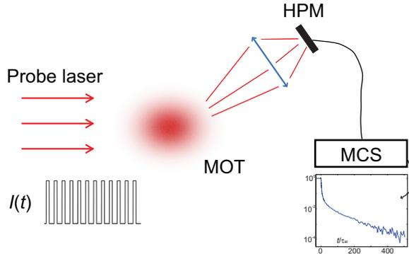
Fig. 1. (color online). Principle of the experiment. A large probe laser illuminates the atomic sample for  $30 \mu\text{s}$  and is switched off rapidly. The fluorescence at  $\sim 35^\circ$  is collected by a hybrid photomultiplier (HPM) and recorded on a multi-channel scaler (MCS). The experiment is repeated 500000 times. At each cycle, 12 pulses are recorded during the free expansion of the cloud, allowing the on-resonance optical depth to vary.
