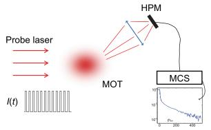
Figure 1 | Principle of the experiment. A large probe laser illuminates the atomic sample for 30  $\mu$ s and is switched off rapidly. The fluorescence at  $\sim 35^{\circ}$  is collected by a hybrid photomultiplier (HPM) and recorded on a multi-channel scaler (MCS). The experiment is repeated 500000 times. At each cycle, 12 pulses are recorded during the free expansion of the cloud, allowing the on-resonance optical depth to vary.
