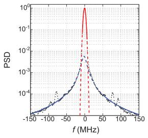
Fig. S4. Spectrum of the probe laser. The power spectrum density (PSD) of a beat-note signal with a reference laser has been averaged 100 times (scanning time  $\sim 1$  s) and the central frequency ( $\sim 1$  GHz) has been shifted to zero (black dots). The result can be fitted by a Gaussian in the central part (red) and by a Lorentzian in the wings (blue).
