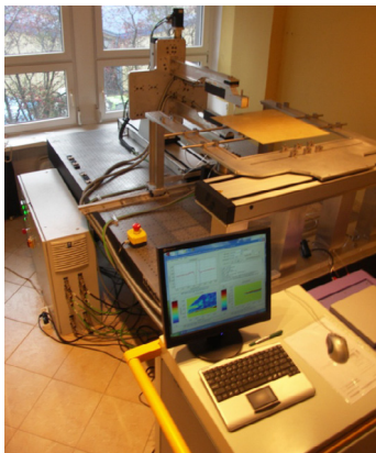
Fig. 2. Terahertz TDS spectrometer with scanning unit.
