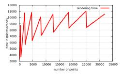
Figure 9: GPU rendering time on an NVIDIA 970M, up to 32000 points. In this case, N=512. The sudden drops correspond to the changes of KDE resolution. One can see that the rendering is bounded by a constant. In practice, with  $n_0=1000$ , there is no more than 16000 points in a 1000\*1000 visualization.
