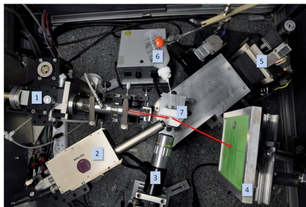
Fig. 2 The in situ monitoring set-up on a rotating anode X-ray generator: 1. X-ray (Mo, \lambda_{\text{K}\alpha} = 0.709 \text{ \AA} ), 2. XRF detector, 3. OM, 4. image plate, 5. translation table, 6. chlorinated solution, 7. cell.
