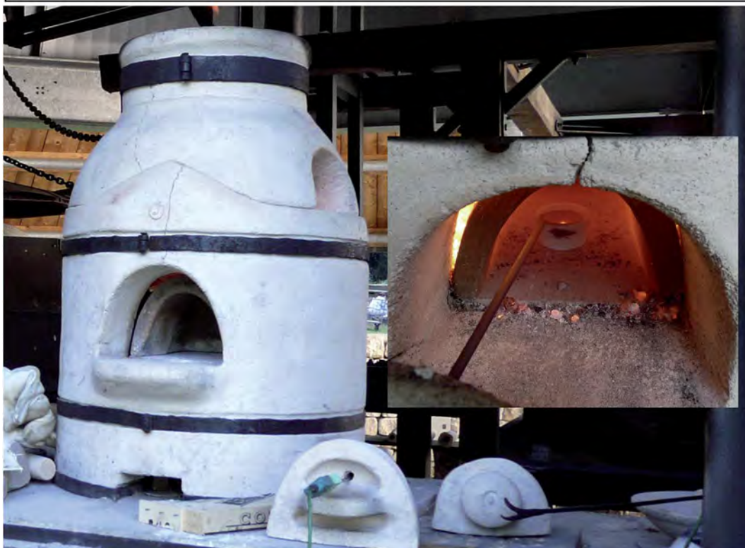
Fig. 1. Flowchart of the experimental cupellation process and experimental furnace used during the experiments.
