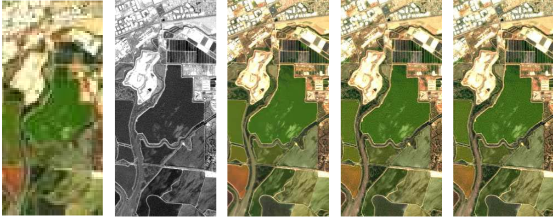
Fig. 4. Hyperspectral pansharpening results. 1st column: HS image. 2nd column: PAN image. 3rd column: Reference image. 4th column: ADMM [23]. 5th column: Proposed method.
