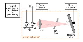
Fig. 1. Experimental setup for measuring velocity of a rotating disk. The disk is tilted around the vertical axis by  $10^{\circ}$  to produce a small velocity component in the direction of the laser beam.
