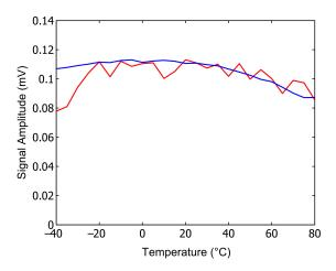
Fig. 6. Dependence of the LV signal strength on temperature: measured (red solid); modelled (behavioural slope efficiency, blue solid).
