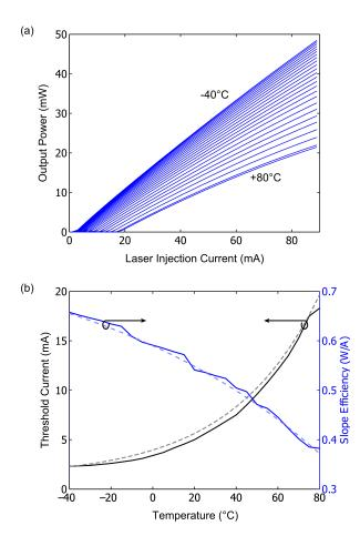
Fig. 2. (a) Output power as a function of laser injection current at different temperatures (in the temperature range from -40 °C to +80 °C in steps of 5 °C), and (b) slope efficiency and threshold current as a function of temperature. Slope efficiency decreases with temperature while injection current threshold increases.
