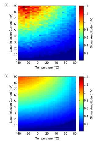
Fig. 7. PD signal strength as a function of the injection current and temperature: (a) Measured, and (b) modelled.
