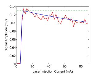
Fig. 4. Dependence of the LV signal strength on injection current: measured (red solid); modelled (constant slope efficiency of an ideal laser diode, green dashed); modelled (behavioural slope efficiency, blue solid).
