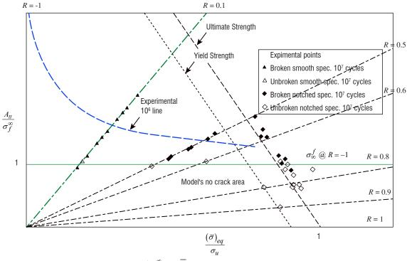
Figure 8 - Experimental multiaxial  $A_{II} / \sigma_f^{\infty}$  vs.  $(\overline{\sigma})_{eq} / \sigma_u$  Haigh diagram of a TA6V alloy at a low temperature
