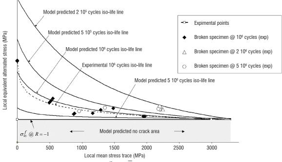
Figure 10 - Partial multiaxial  $A_{II} / \sigma_f^{\infty}$  vs. tr $\overline{\sigma}$  Haigh diagram (TA6V alloy at a low temperature).
