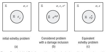
Figure 2 - a) Initial Eshelby problem of an inclusion with free strain  $\varepsilon_F$ , b) Considered problem with matrix plasticity and damaged inclusion, c) Problem making both cases a) and b) equivalent, due to an adequate choice of the free strain  $\varepsilon_F^*$ .
