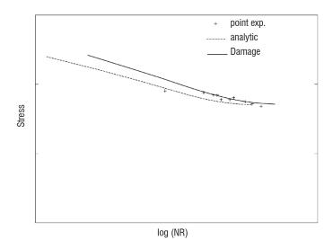
Figure 3 - Illustration of Stages 4 and 5 of the identification procedure on the Wöhler curve for TA6V at a low temperature (marks: experimental, analytical: Eq. (20), DAMAGE: numerical solution by DAMAGE\_EAS of set of equations (8) and (11)).
