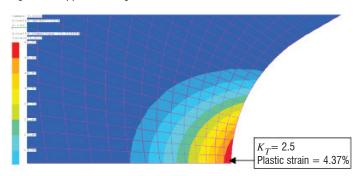
Figure 6 - Maps of plastic strain after pre-plastification for one of the  $K_T = 2.5$  specimens (applied load ratio  $R_F = F_{min} / F_{Max} = 0.88$ , computed stress ratio  $R = \sigma_{min} / \sigma_{Max} = 0.72$ ).
