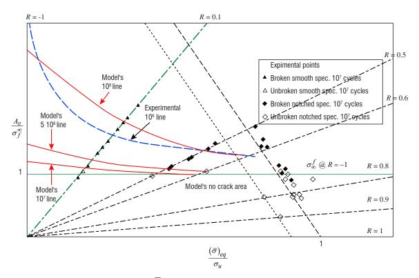
Figure 9 - Multiaxial  $A_{II} / \sigma_f^{\infty}$  vs.  $(\overline{\sigma})_{eq} / \sigma_u$  Haigh diagram with two-scale damage model iso-lifetime lines
