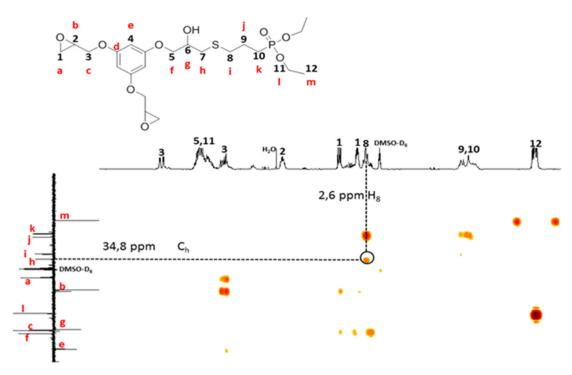
Fig. 1. HMBC 2D <sup>1</sup>H-<sup>13</sup>C NMR spectrum of the diglycidyl thiophosphonated phloroglucinol (P2EP1SP) in DMSO-d<sub>6</sub>.
