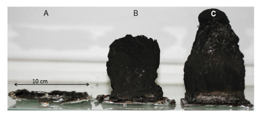
Fig. 9. Pictures of the cone residues: DGEBA-IPDA (A), 3% P3SP (B) and 3 %P P2EP1SP (C) thermosets obtained by cone calorimeter.
