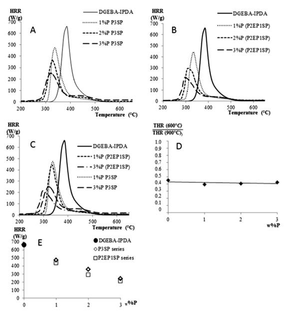
Fig. 7. PCFC curves of the P3SP-containing thermosets (A), P2EP1SP-containing (B) thermosets compared to the P-FR-free DGEBA-IPDA and comparison of P3SP vs P2EP1SP-containing (C) thermosets, (THR<sub>600</sub>/THR<sub>900</sub>) obtained by PCFC at 1 °C/s on P3SP-containing thermoset (D) and pHRR vs phosphorus content (E).
