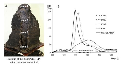
Fig. 10. PCFC curves of the cone calorimeter residue at different heights of the 3%P(P2EP1SP) thermoset obtained at 1 °C/s.
