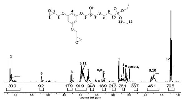
Fig. 2. <sup>1</sup>H NMR spectrum of the diglycidyl thiophosphonate phloroglucinol (P2EP1SP) in DMSO-d<sub>6</sub>.
