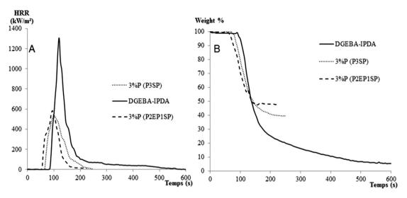
Fig. 8. Heat release rate curves (A) and mass monitoring curves (B) of the 3 w%P-containing thermosets obtained with cone calorimeter at an irradiance of 35 kW/m<sup>2</sup>.
