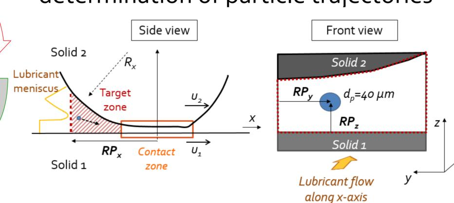
Considering a contaminated lubricant supposes to take into account both the lubricant behavior and the particles dynamics.
