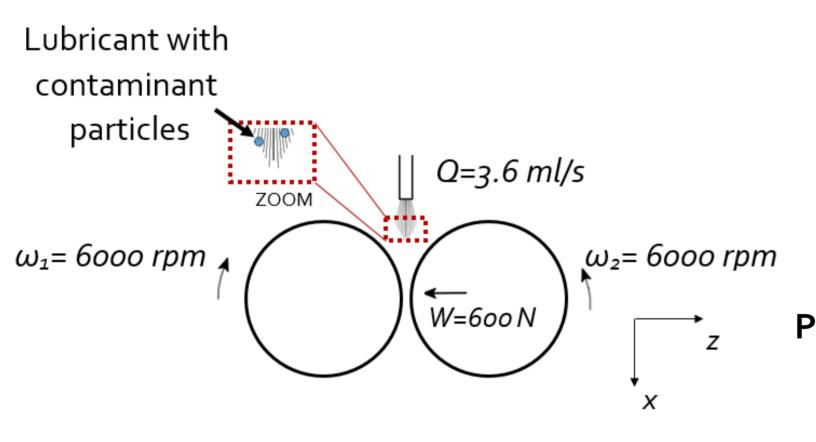
Tests with the twin-disc machine and the contamination test bench:
