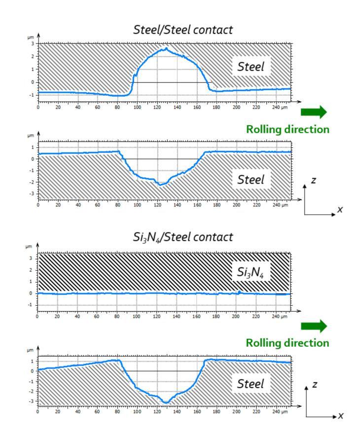
Tests with different couples of materials
