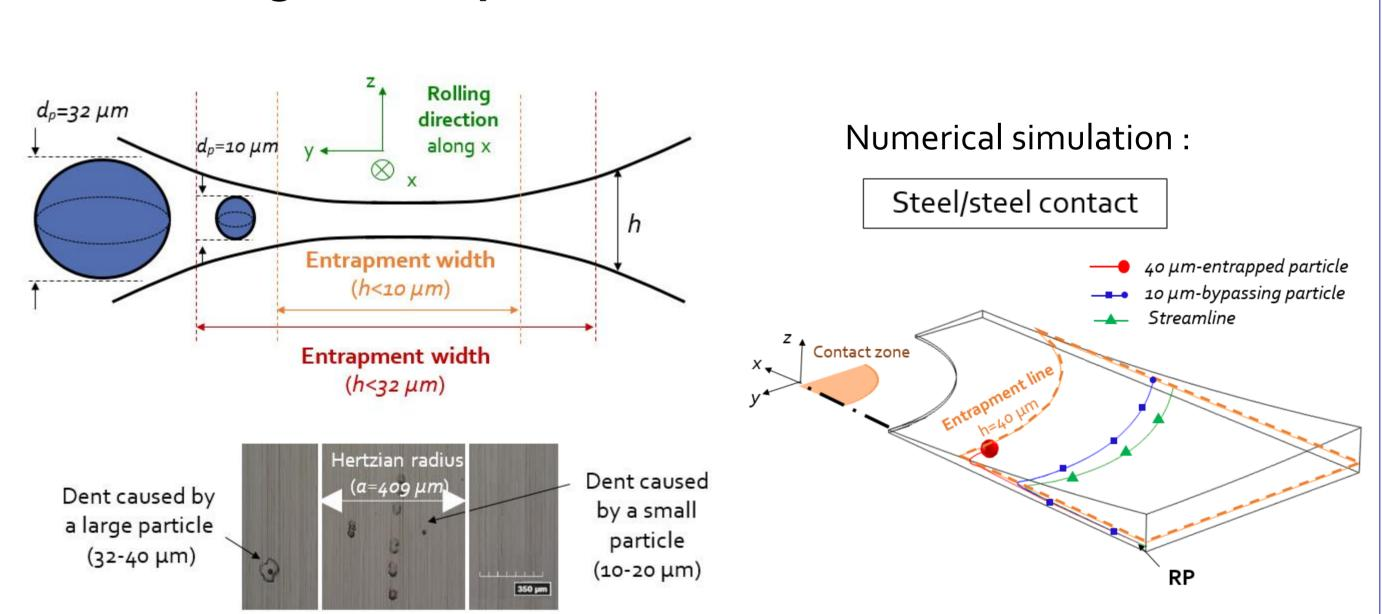
Larger particles are more likely to be entrapped, in accordance with<sup>2</sup>, due here to a larger entrapment width.
