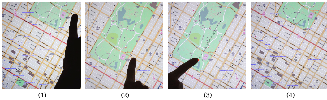
Fig. 5. Panning a map on a tabletop. (1-2) The user swipes on the touch screen to set the viewport over the region of interest on the map, revealing more of Central Park in New York City. (3-4) She touches the screen and remains still to invoke Dwell-and-Spring on the map and go back to her view on Midtown.
