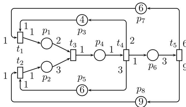
Fig. 3. Modeling an assembling line using a TWEG.
