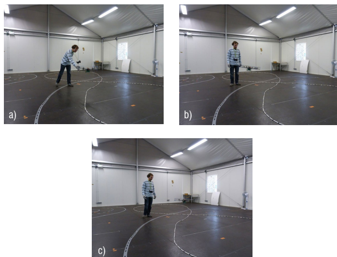
Figure 9 - The quadrotor is moved from its initial path by a manual perturbation. It can retrieve the followed line
