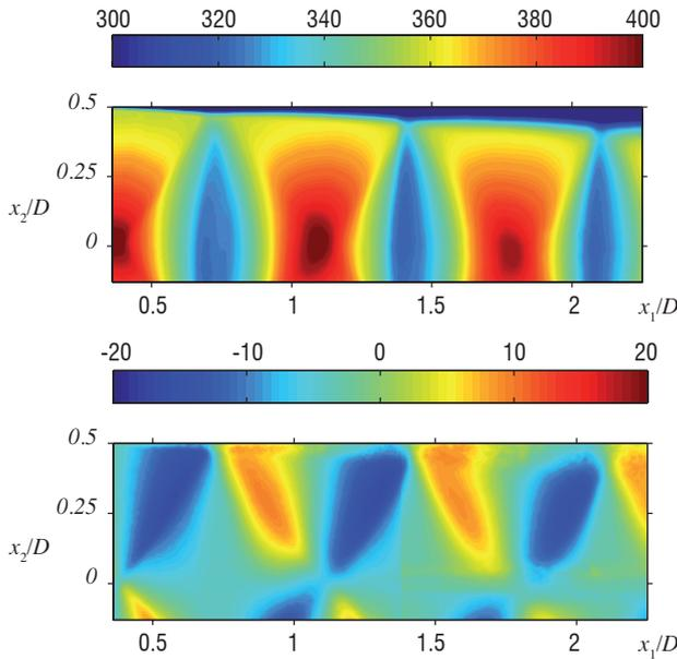
Figure 2 - Measured longitudinal (top) and transverse (bottom) mean velocity field (color scale in  $\text{m}\cdot\text{s}^{-1}$ ) in a plane containing the jet axis for  $M_j = 1.15$ , with a notched convergent nozzle and an additional slow coflow at  $M_j = 0.05$  to ensure seeding of the supersonic jet surroundings. The PIV set-up leads to about 190 velocity vectors over one jet diameter. More details regarding the quality checks can be found in André [5,10].
