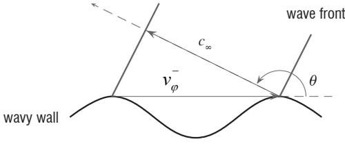
Figure 5 - Generation of Mach waves by a wavy wall moving at supersonic phase speed  $u_c$ , the direction of the radiation  $\cos \theta = c_\infty / v_\phi$  is obtained by matching the velocity trace along the flow direction. There is an analogy with the acoustic radiation of a vibrating plate for the reader familiar with vibroacoustics.
