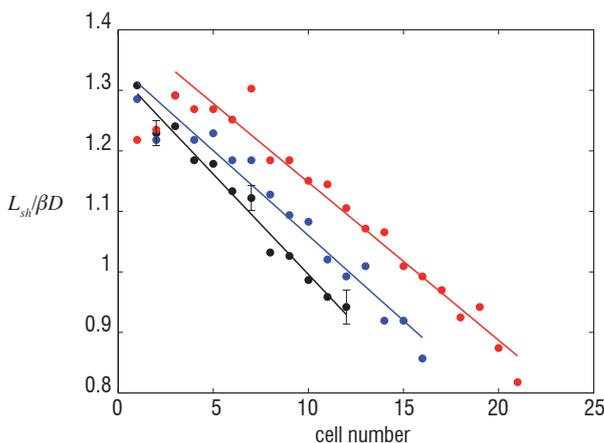
Figure 9 - Individual shock cell length  $L_{sh}$  normalized by  $\beta D$  as a function of the cell number and for three flight Mach numbers, •  $M_f = 0$ , •  $M_f = 0.22$ , •  $M_f = 0.39$ . The experimental data are obtained from Schlieren visualizations for the  $M_f = 1.10$  jet [5,9].
