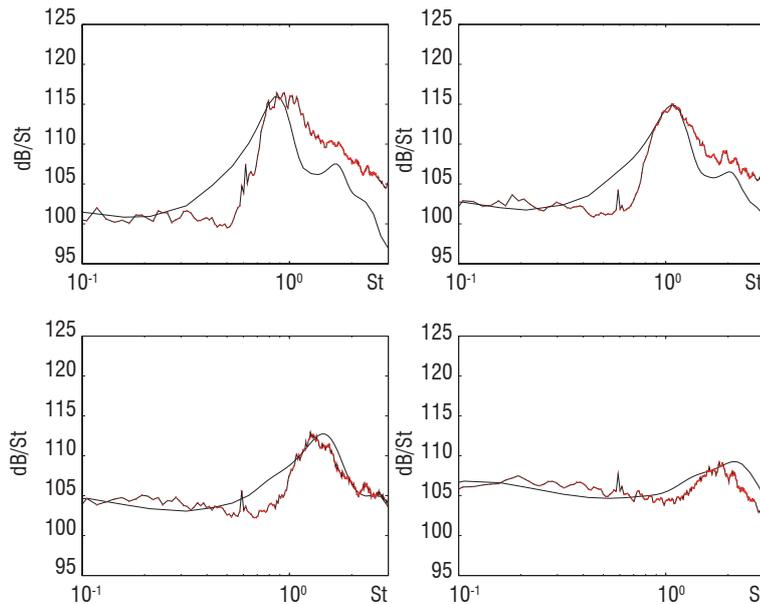
Figure 7 - Acoustic spectra in dB/St as a function of the Strouhal number  $St = fD/u_j$ , of the  $M_j = 1.15$  jet for an observer angle  $\theta = 130^\circ, 110^\circ, 90^\circ$  and  $70^\circ$ ; —•— measurements [5], — predicted BBSAN component [15], which is expected to dominate in the rear quadrant. The observer angle  $\theta$  is taken from the downstream jet axis.
