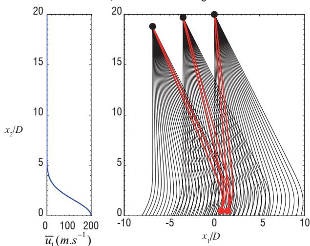
Figure 10 - Illustration of ray-tracing in the direct and adjoint problems, • observer positions, • source, — adjoint ray to the source domain at a given  $\mathbf{x}$ , — direct ray from the source  $\mathbf{y}$  to the observer location  $\mathbf{x}$ .
