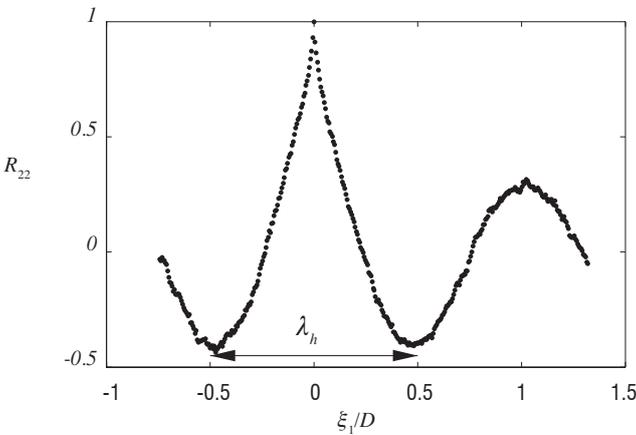
Figure 4 - Correlation function  $R_{22}$  measured by PIV at  $x_1 = 3D$  along the lip line ( $x_\perp = D/2$ ) for a screeching  $M_j = 1.10$  jet, as a function of the axial separation  $\xi_1$  normalized by the nozzle diameter. The length wave  $\lambda_h = u_c / f_s \approx D$  can be identified with  $u_c = 0.65u_j$  and  $f_s = 5870$  Hz.
