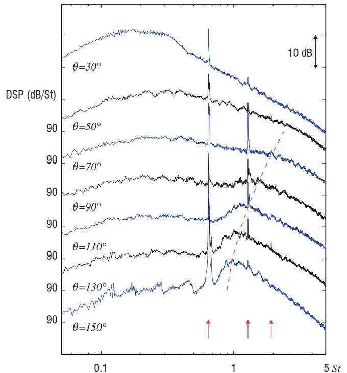
Figure 3 - Narrow-band acoustic spectra of  $M_j = 1.10$  jet, measured at  $r/D = 53.2$  as a function of the Strouhal number  $St$ , and for different angular positions. The angle  $\theta$  is taken from the downstream jet axis. The red dashed line corresponds to relation (7) and the red arrows indicate the fundamental screech frequency and its two first harmonics. Data from André [5].
