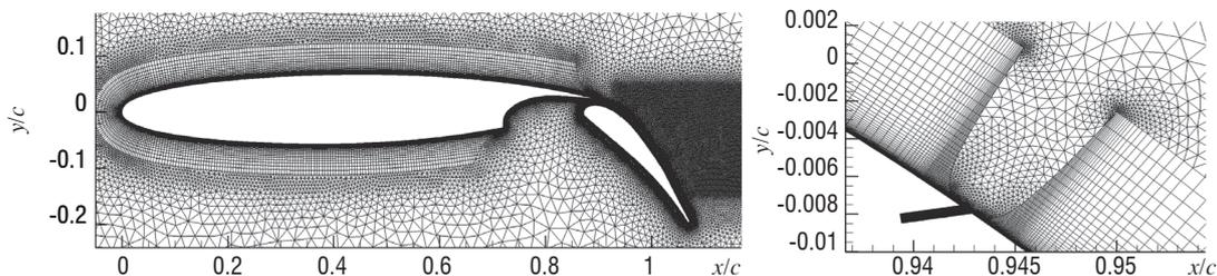
(a) two-dimensional grid for the DLR-F15 airfoil with single-slot-actuator
