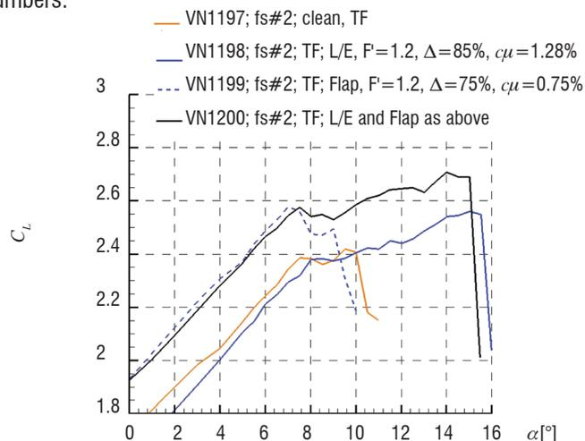
Figure 4 - The maximum lift improvements by vortex generator jets applied at the wing leading edge and single slot pulsed blowing at the trailing edge flap ( $M=0.15$ ,  $Re=2 \times 10^6$ ,  $T=290K$ , atmospheric wind tunnel testing)
