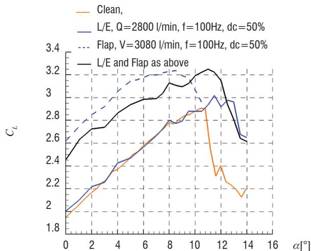
Figure 5 - The maximum lift improvements at high Reynolds number by vortex generator jets applied at the wing leading edge and multi-slot pulsed blowing at the trailing edge flap ( $M=0.15$ ,  $Re=4.2 \times 10^6$ ,  $T=170K$ , cryogenic wind tunnel testing).
