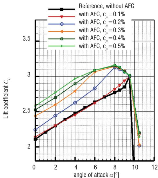
Figure 11 - Lift coefficient over the angle of attack for the DLR-F15 airfoil from URANS simulations, with and without AFC, according to [13]; configuration: 2eOpt49; inflow conditions:  $M=0.15$ ,  $Re=2 \times 10^6$
