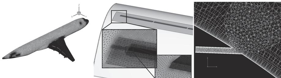
(c) three-dimensional grid for a wing-body configuration with 21 slot-actuators
